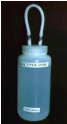
Figure 4-3. Loop and mercury sample bottles
