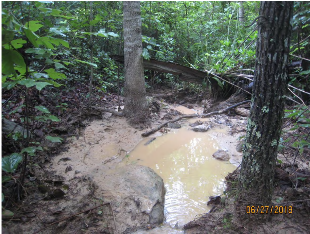
Photo 1: Sedimentation within “SMM-15” ~160’ downstream of LOD; Depth = 3”
