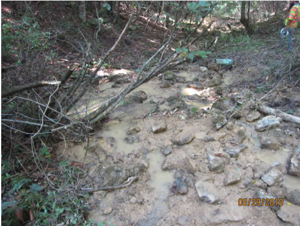
Photo 3: Sediment in stream approximately 300' downstream of ROW; Depth = 1-3" Orientation: Downstream
