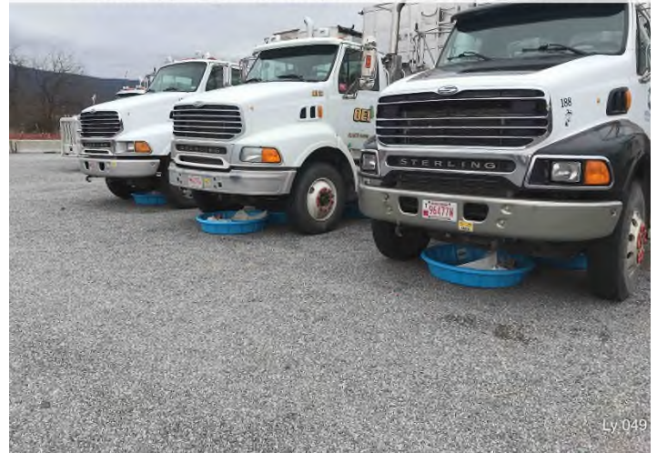
Figure 4: Laydown Yard 049 – Drip pans installed and properly functioning on stored equipment.
