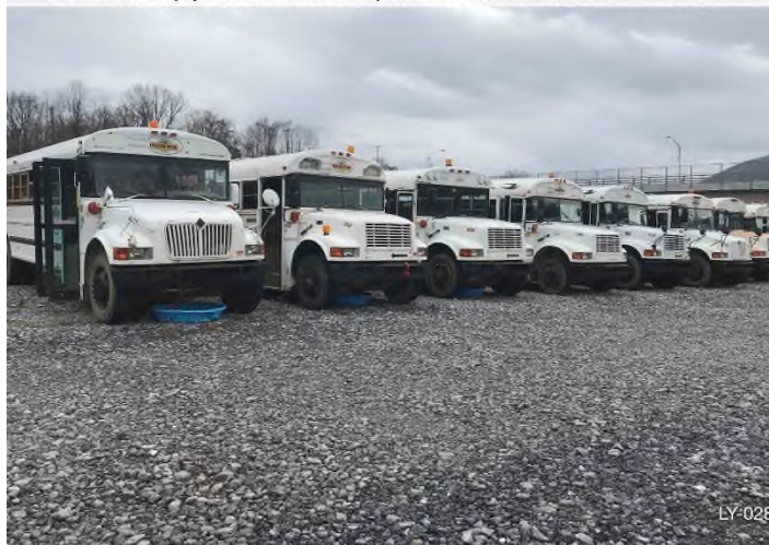
Fig. 4: Laydown Yard 028 – Secondary containment placed under equipment storage to contain potential leaks.
